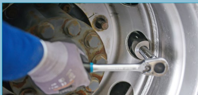
Rotate the spindle drive size 17 until the outside rim disengages from the inner rim
