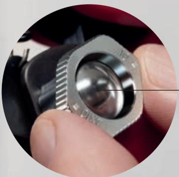
The crimping pliers can be adjusted to large wire ferrules of 16 mm<sup>2</sup> or 2 x 10 mm<sup>2</sup> with the adjusting wheel.
