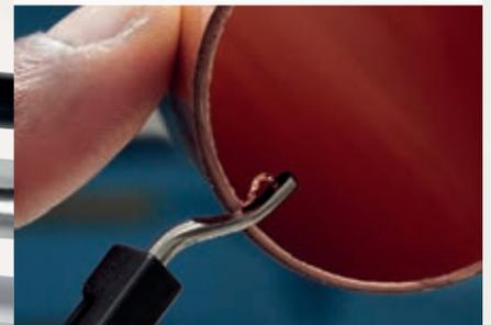
The precisely ground deburring tool can be taken out of the tool when needed.
