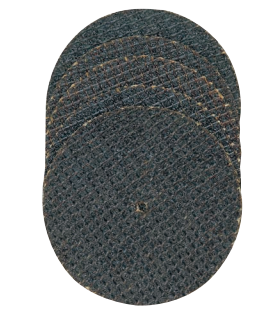
NO 28 819 20 pieces The cutting discs are available in \varnothing 22 x 0.8 and \varnothing 38 x 1. Nearly unbreakable, making them usable to remove stock. Will cut alloyed, standard and stainless steels, non-ferrous metals and even wood and plastic. Arbor shaft of \varnothing 2.35.
